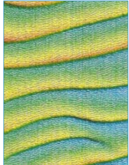
MULTIBEAM RECORD IN A SANDWAVE AREA WITH TRAWLING SCARS, 6 METERS APART.
